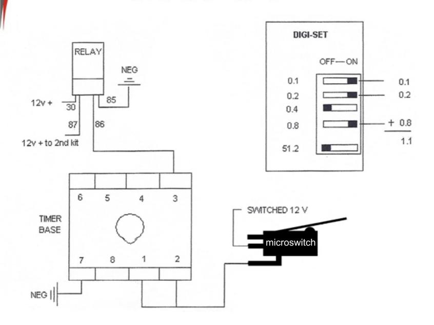
This time delay switch is set to activate after a delay of 1.1 seconds.
