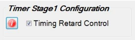
**Stage1 Timer, Timing Retard Control** - this setting configures the Stage1 Timer, +12V output to be On whenever Stage1 Nitrous is On (Solenoids functioning). Check to enable.
