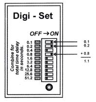
This time delay switch will allow you to activate/deactivate a stage of nitrous as a function of time.
