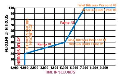
Nitrous Delay Timer = 1.000 seconds Starting Percent = 20% Final Nitrous Percent #1 = 40% Nitrous Build Time #1 = 4.000 seconds Final Nitrous Percent #2 = 100% Nitrous Build Time #2 = 2.000 seconds
