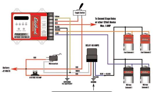
An optional RPM window switch may be connected here. Any RPM switch with a ground control output may be used.
