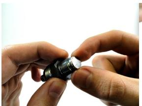
Shown above is the new burst disc being installed correctly on the racer safety. Be sure when installing the burst disc that you do not collapse the sides of the disc or damage the disc in any way.
