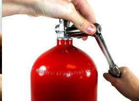
Hand tighten the racer safety into the bottle valve assuring that it seats correctly and the burst disc remains in place. Once hand-tight, **torque to 17 ft. lbs.** using a properly calibrated torque wrench.
