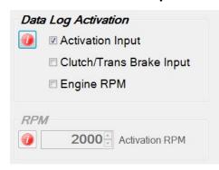
Data Log Activation - these settings determine when the controller begins recording data.
