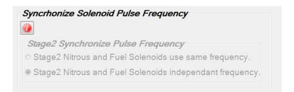
**Stage2 Synchronize Pulse Frequency** - the Stage2 nitrous and fuel solenoids can be configured to function at the nitrous solenoid frequency (hertz) only (both Stage2 outputs synchronized). Or the Stage2 nitrous and fuel solenoid output frequencies (hertz) may be set independently.
