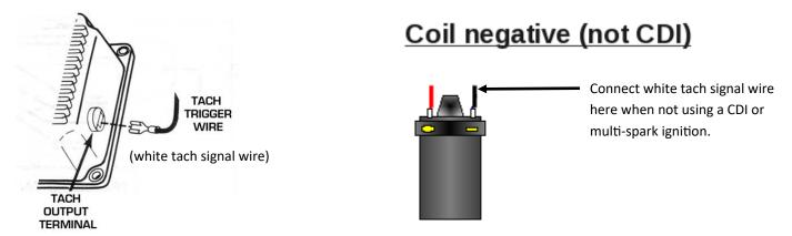
The tach input signal can also be connected to a +5 volt or +12 volt square wave signal on newer fuel injected vehicles. You will need to research the vehicle in question and check to see if the ECM provides a tach (rpm) signal. You may also purchase an aftermarket tach signal adapter if needed.
